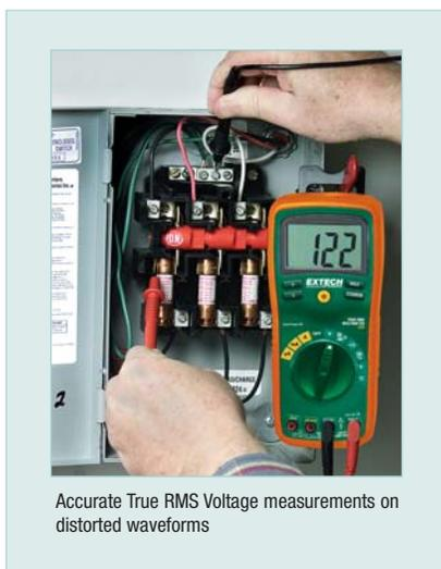
Accurate True RMS Voltage measurements on distorted waveforms
